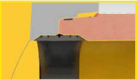
2 Connector connection of PERFECT Pipe to the lined manhole base
