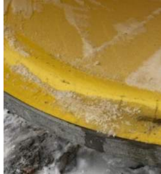
Ice build up on inside of the spigot
