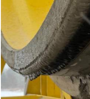
Ice built-up and freeze the low transmission ring
